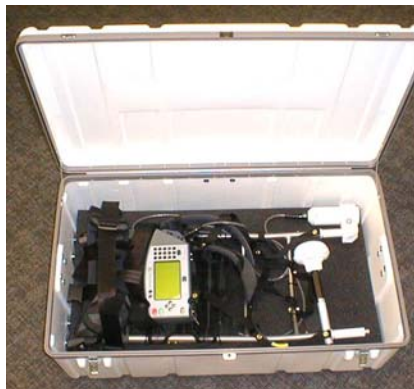
G-859 and GPS Re-Usable Shipping Case with foam padding and transport wheels
