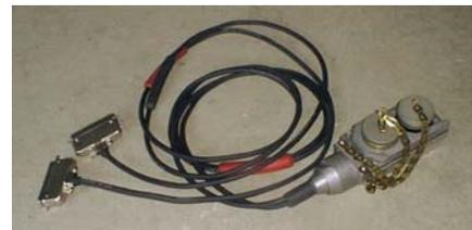
Geophone cables and a variety of adapters are available to interface to geophone cables and seismographs. Contact factory for information.
