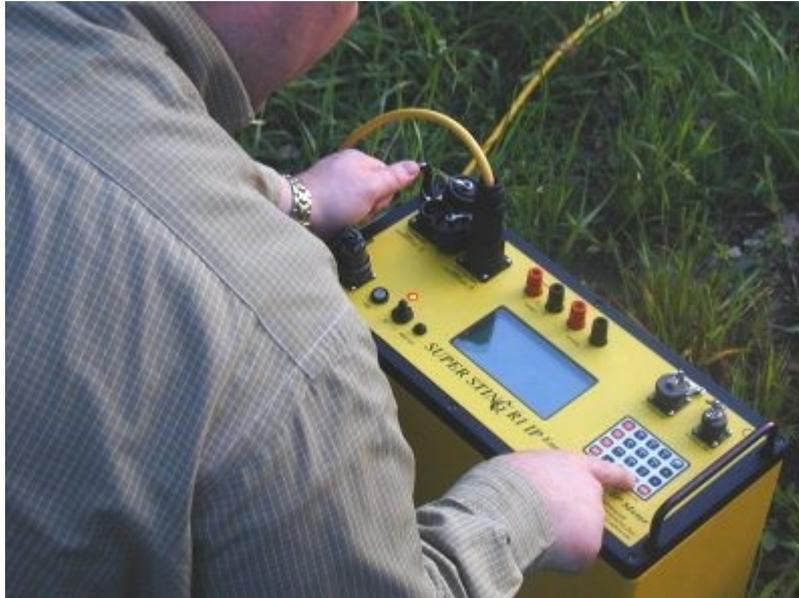
The **SuperSting R1 IP** is a state-of-the-art single-channel portable memory earth resistivity meter with memory storage of readings and user defined measure cycles. It provides the highest accuracy and lowest noise levels in the industry.
