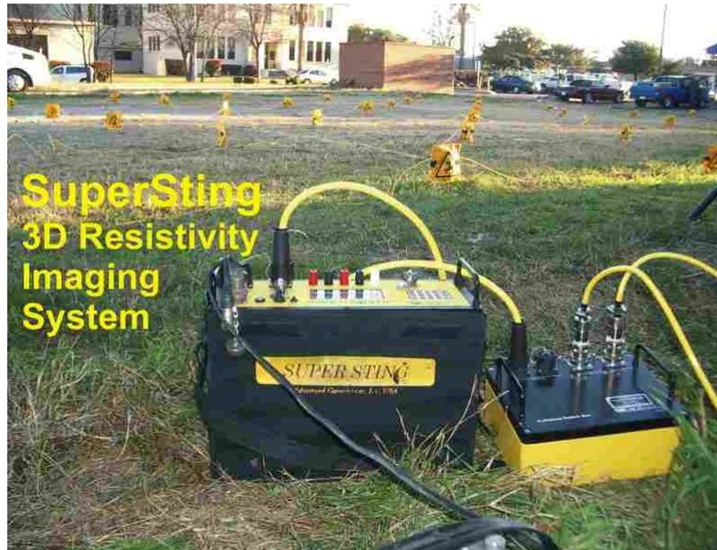
The **SuperSting R8 IP** is a state-of-the-art multi-channel portable memory earth resistivity meter with memory storage of readings and user defined measure cycles. It provides the highest accuracy and lowest noise levels in the industry.
