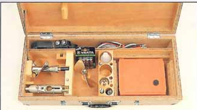
Fig. 2: Instrument case for a current meter used on rod
