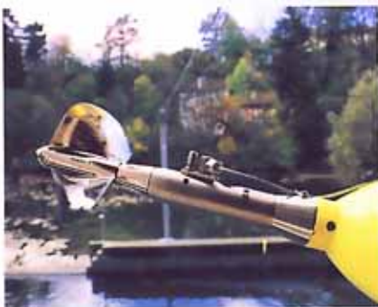
C 31 Cable suspended current meter on gas spring tensioned cable-way.
