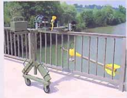
C 31 with 25 kg Single-drum winch and movable Trolley for the measurement e.g. from a bridge.
