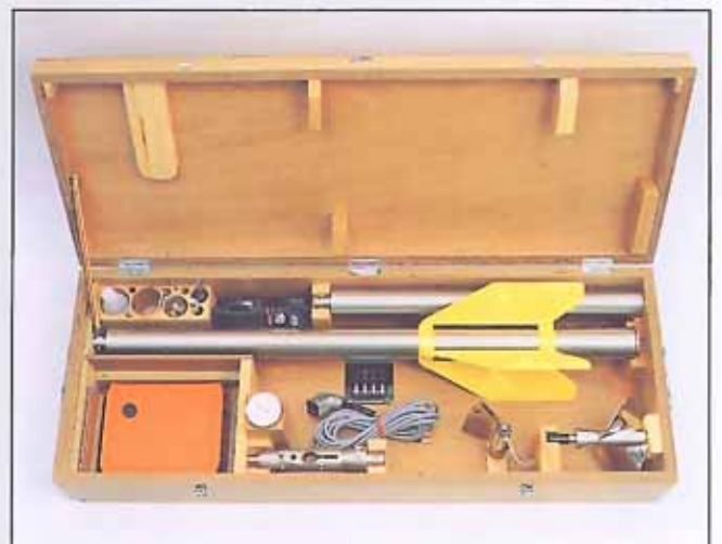
Fig. 8: Instrument case for C 31 cable-suspended meter equipment with middle piece 25 kg, 50 kg or 100 kg.
