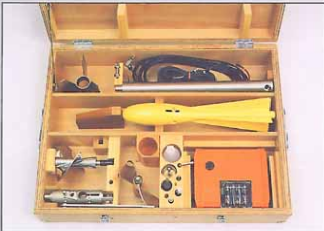
Fig. 5: Instrument case for cable-suspended meter equipment with sinker.
