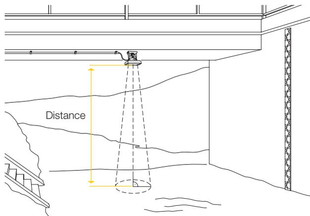
The time from transmission until reception of the reflected pulse (time delay) is longer the further the OTT RLS is from the water surface and thus the lower the water level. This correlation is used by the OTT RLS to determine the time delay and calculate the distance to the water surface (distance value).
