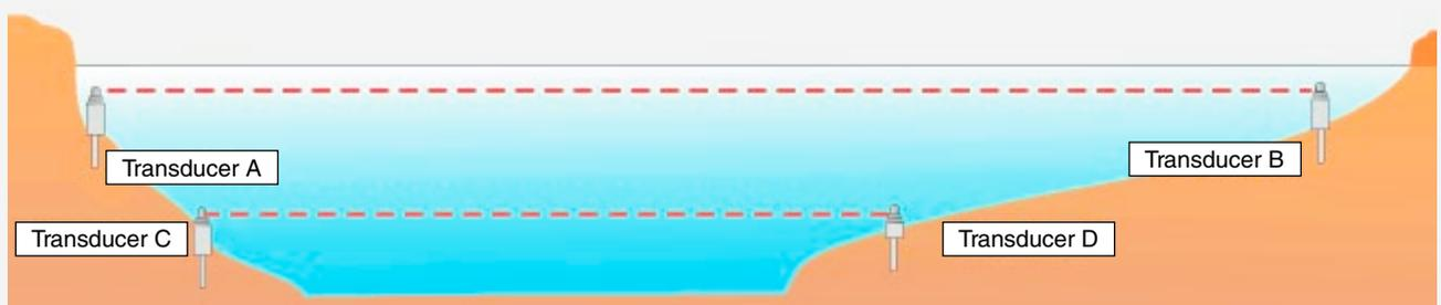
\*) "Two-path cross arrangement with responder" currently being developed
