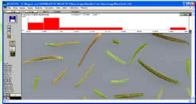
The Pro version can classify seeds and needles in groups based on their color (brown and green as in the sample above or different brownish tint as in the example to the left) and analyse them separately. It can also quantify the area occupied by each color for disease or insect damage analysis. Very subtle color differences can be detected. For color analysis, a scanner is recommended as image acquisition device.
